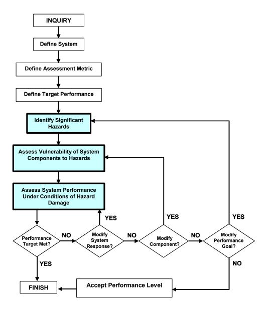
Figure 1-1 Decision-making Process for Assuring System Performance Goals Are Met
