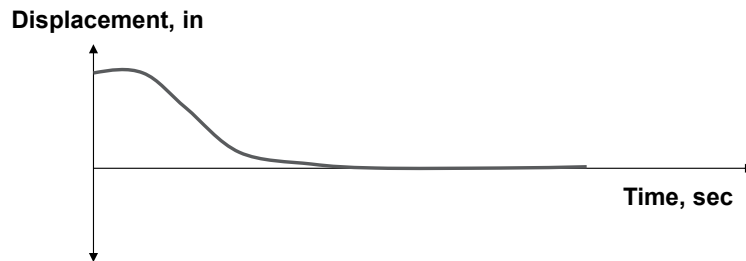
Response of Critically Damped System, \xi=1.0 or 100% critical
