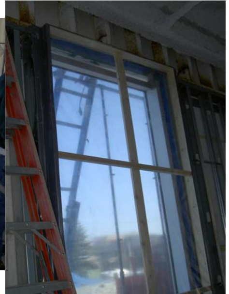
Figures 12 and 13: Field-testing of water penetration to ASTM E 1105 with spray rack.
