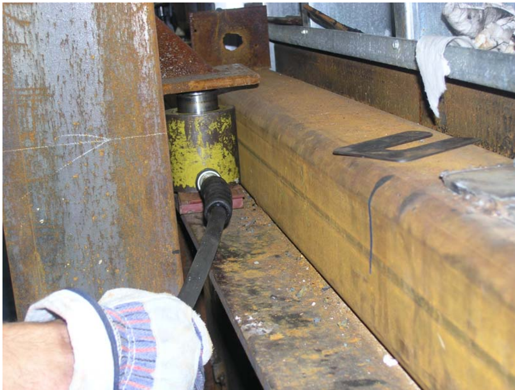
Figure 4 Installing hydraulic jacks to simulate inter-story drift.
