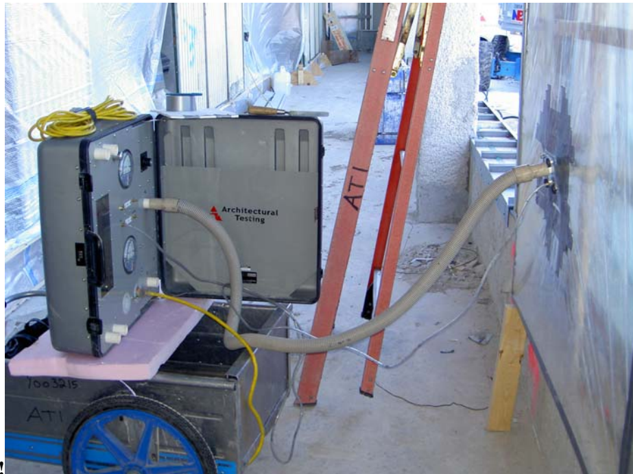
Figure 11 ASTM E 783 test with exterior chamber, testing a window and its perimeter window-to-wall joint
